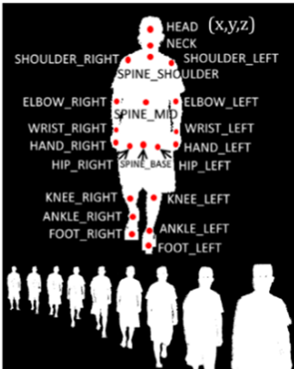
Fig. 4 3D coordinates of 21 joints (in the upper area) and the corresponding silhouette images (in the lower area) in our dataset
