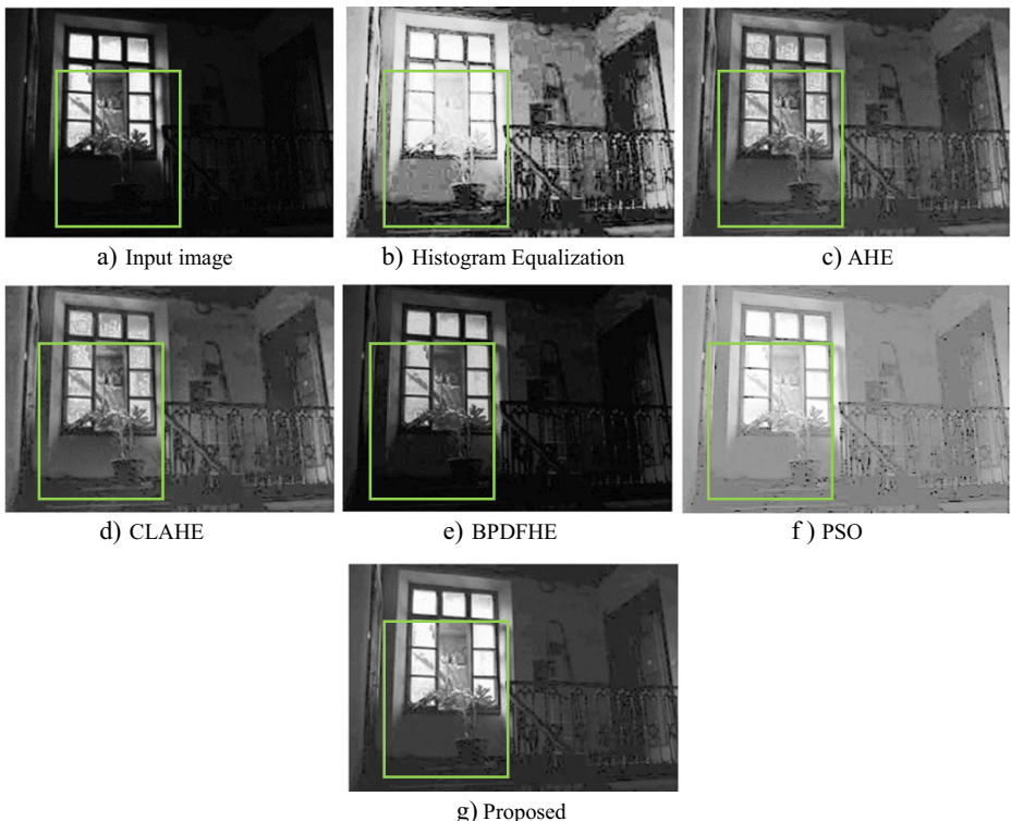
Fig. 3 Enhanced ‘House image’ using various contrast enhancement techniques
