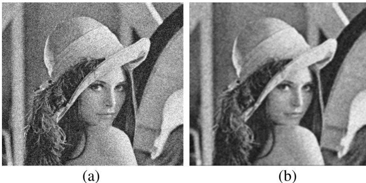
Fig. 2 (a) Noisy image with Gaussian noise \sigma = 25 . (b) Filtered image with semi-soft thresholding
