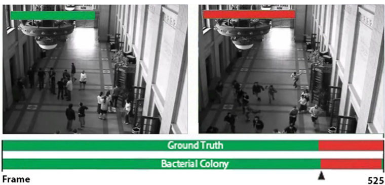
Fig. 13 Detection by Kohonen network with data from bacteria colony behavior
