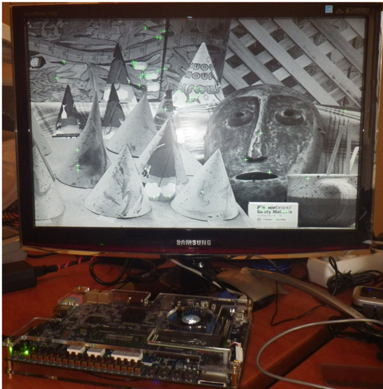
Fig. 8 Verification of the proposed architecture using the DE2i-150 development board
