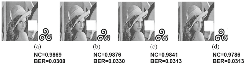
Fig. 30 Result under cropping attack(128 × 128) and recovered watermark image using a 20 division b using 30 division c using 40 division d using 50 division
