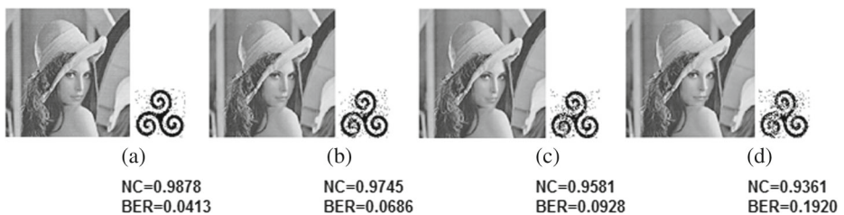
Fig. 19 Result under Gaussian Low pass filtering ( 3 \times 3 ) attack and recovered watermark image using a 20 division b using 30 division c using 40 division d using 50 division
