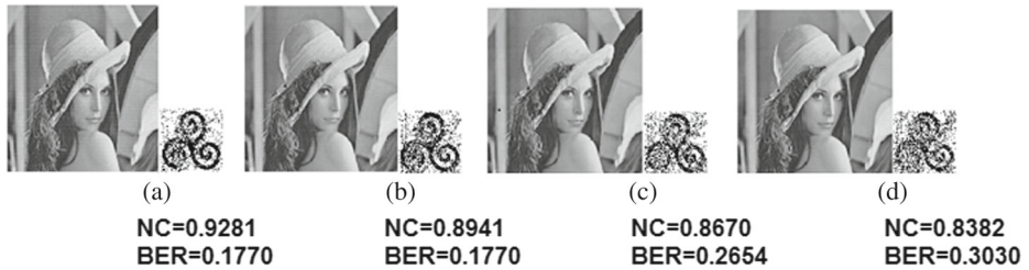
Fig. 18 Result under Gaussian Low pass filtering ( 2 \times 2 ) attack and recovered watermark image using a 20 division b using 30 division c using 40 division d using 50 division
