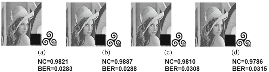
Fig. 29 Result under cropping attack(128 × 128) and recovered watermark image using a 20 division b using 30 division c using 40 division d using 50 division
