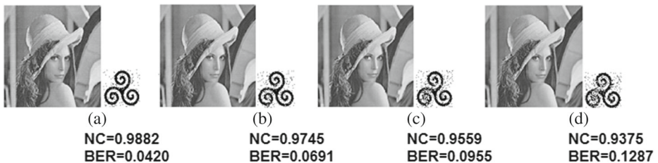
Fig. 21 Result under Gaussian Low pass filtering( 7 \times 7 ) attack and recovered watermark image using a 20 division b using 30 division c using 40 division d using 50 division
