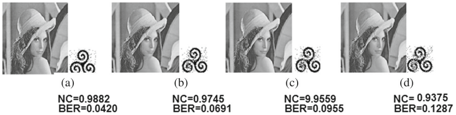
Fig. 20 Result under Gaussian Low pass filtering ( 5 \times 5 ) attack and recovered watermark image using a 20 division b using 30 division c using 40 division d using 50 division
