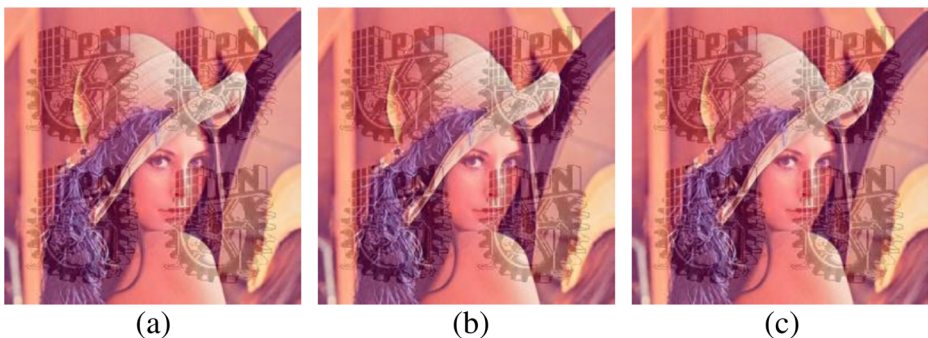
Fig. 12 Images obtained after performing the collusion attack. Images a , b and c show the results by averaging 10, 20 and 40 different versions of dual watermarked images respectively
