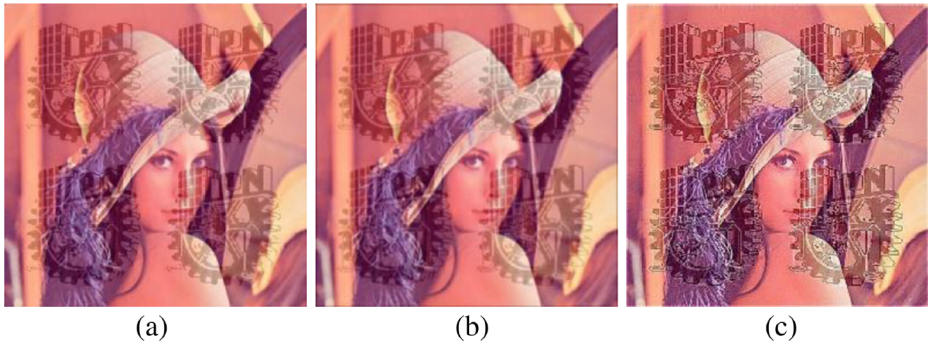
Fig. 11 Images obtained after performing some common image processing techniques to the dual watermarked images. Images a , b and c show the results for the 3 \times 3 median filtering, 3 \times 3 image smoothing and Laplacian image sharpening attacks respectively
