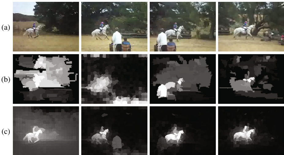
Fig. 1 An example of visual comparison between image-based and video-based salient object detection. a Video frames. b Result of image-based salient object detection by applying [7] independently on each video frame. c Result of video-based salient object detection by using our method
