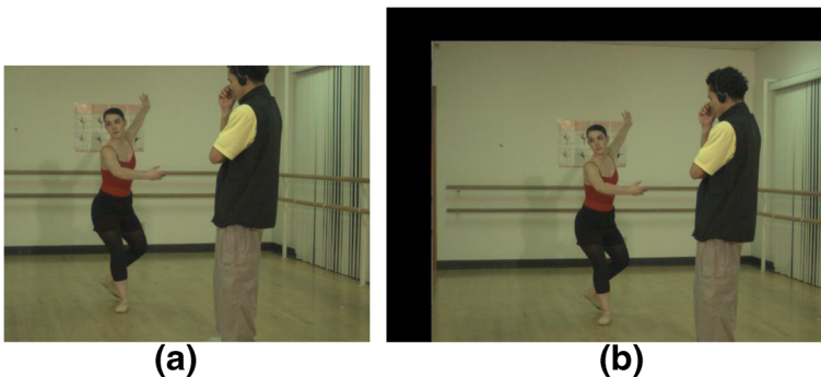
Fig. 18 (a) Distorted image ( 618 \times 821 ) after a cropping attack with a cropping factor of 20, (b) Distorted image ( 1024 \times 768 ) after a translation attack with a translation factor of 10
