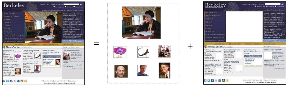
Fig. 1 A Web page ( left ), its dynamic part ( middle ), and its static part ( right )
