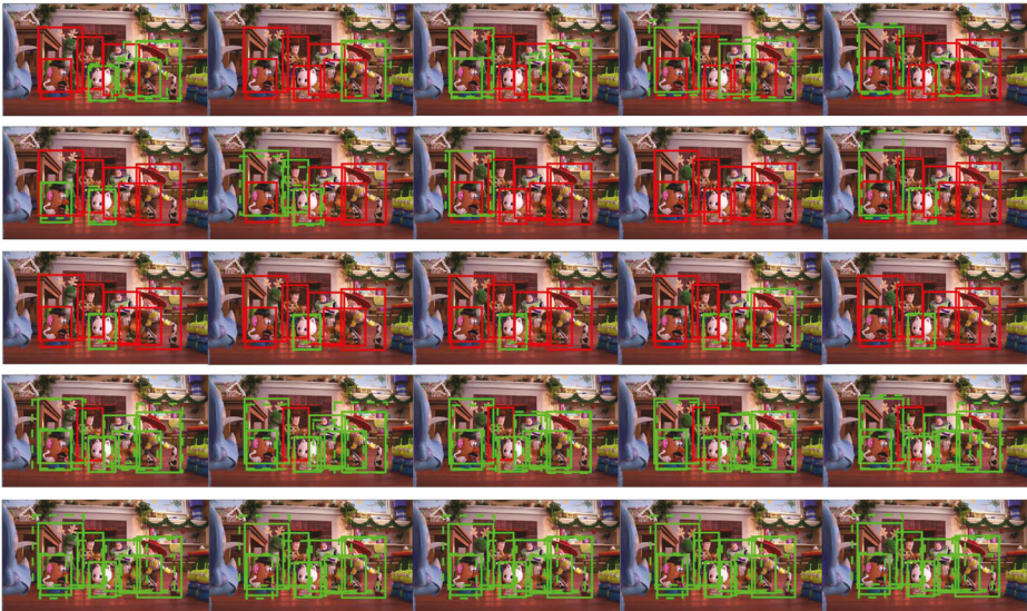
Fig. 4 Comparisons of spatio-temporal bounding box proposals for 5 sequential frames from one shot of our dataset. These proposals are generated by Rahtu [45], Objectness [2], Bing [9], Edgebox [68] and our method from the first line to the fifth line. Green solid rectangles are the annotated ground truths, while green dashed rectangles are the hit proposals. The red solid rectangles are the missed ground truths. ( \alpha = 0.7 and #WIN=1000)
