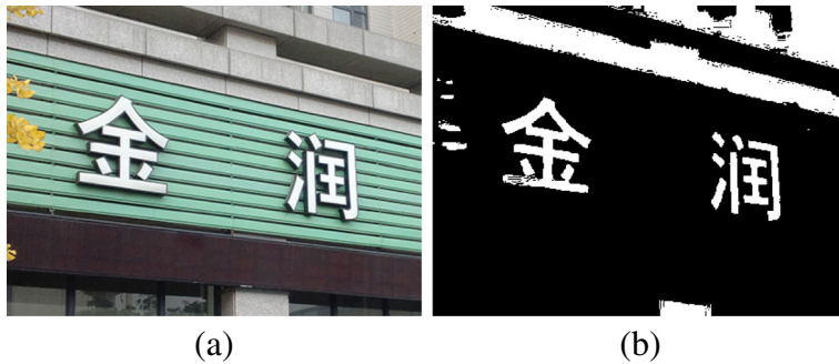
Fig. 9 a An image with characters. b Segmentation results
