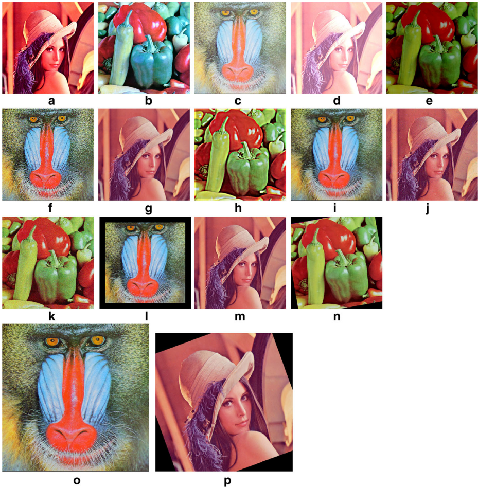
Fig. 3 The attacked watermarked images under attacks. a contrast adjustment ( SSIM = 0.7283 ); b histogram equalization ( SSIM = 0.6642 ); c gamma correction ( SSIM = 0.8541 ); d brighten ( SSIM = 0.7639 ); e darken ( SSIM = 0.5327 ); f sharpening ( SSIM = 0.5650 ); g Gaussian low-pass filtering ( SSIM = 0.8931 ); h Butterworth high-pass filtering ( SSIM = 0.8428 ); i median filtering ( SSIM = 0.7234 ); j salt & pepper noise ( SSIM = 0.7648 ); k Gaussian noise ( SSIM = 0.3858 ); l cropping ( SSIM = 0.7474 ); m JPEG ( SSIM = 0.9884 ); n rotation ( SSIM = 0.8187 ); o scaling ( SSIM = N/A ); p rotation + scaling ( SSIM = N/A )
