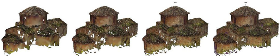
Fig. 5 The four model Representations used in our streaming evaluations. From left to right: Representation 1: 8000 faces, Representation 2: 40,000 faces, Representation 3: 100,000 faces, Representation 4: 360,000 faces
