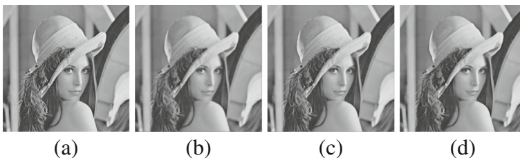
Fig. 2 An original image (a), and its (b) 5 \times 5 average filtered version, 5 \times 5 Gaussian filtered ( \sigma = 1 ) version and (c) 5 \times 5 median filtered version
