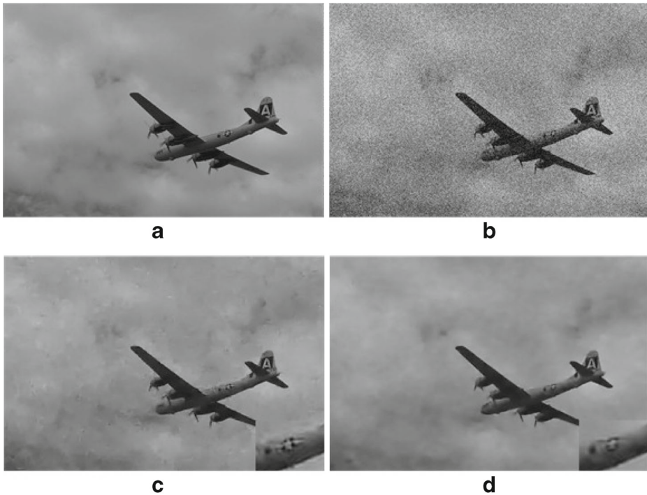
Fig. 1 Denoising results on Test1 image, a-b Original and noisy images, respectively. c-d Denoising results of EPLL and proposed method, respectively
