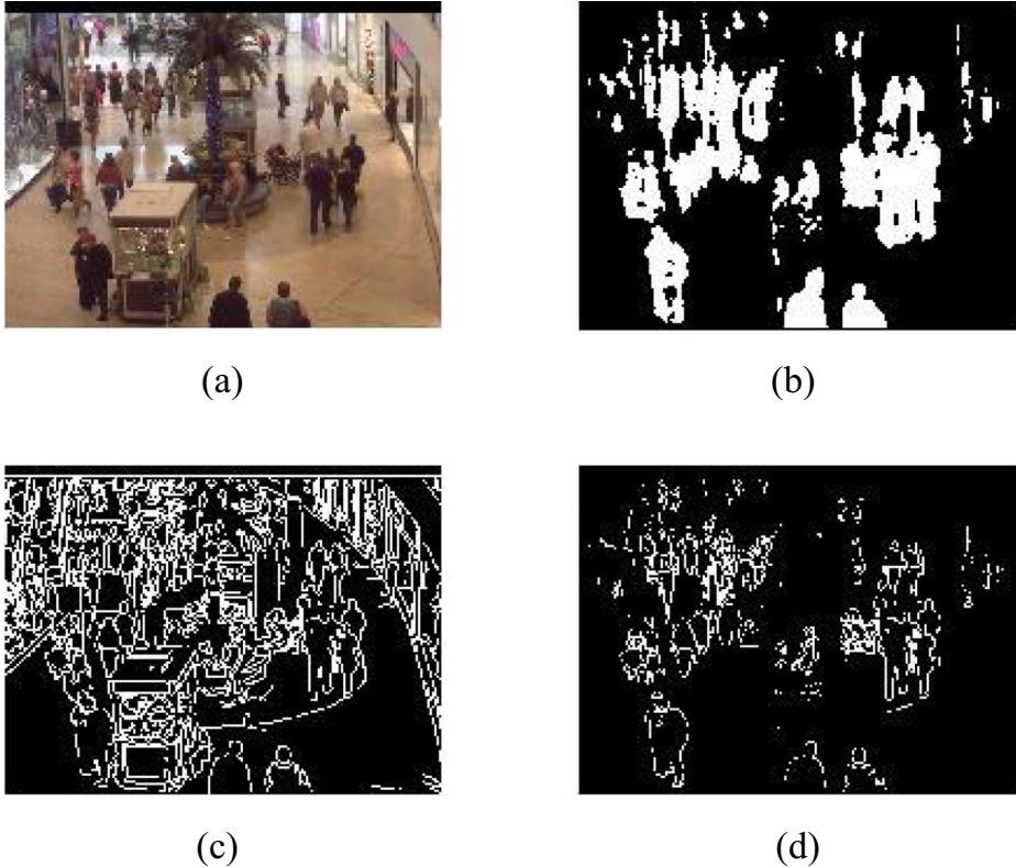
Fig. 6 a An example of the Mall dataset form; b foreground, using GMM algorithm; c edge using Canny detector; d the motion edge, using logical ‘AND’
