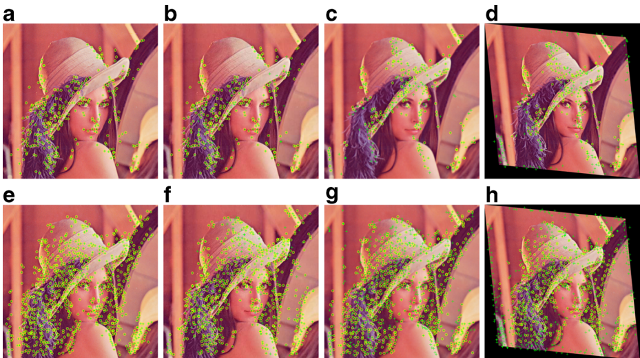
Fig. 1 The feature point detection results using SURF detector and our probability density-based SURF detector (Lena): a SURF detector and no attack, b SURF detector and JPEG compression (QF = 50), c SURF detector and image blurring (1.0), d SURF detector and viewpoint change (10°), e Probability density-based SURF detector and no attack, f Probability density-based SURF detector and JPEG compression (QF = 50), g Probability density-based SURF detector and image blurring (1.0), h Probability density-based SURF detector and viewpoint change (10°). Note: yellow circle denotes the repeated feature points, red plus denotes the detected useful feature points
