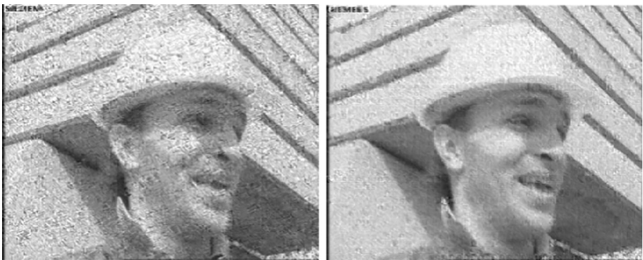
Fig. 3 Visual quality comparison of CS recovery on the 6th frame with subrate = 0.4. From left to right: the KSVD-CS recovered frame; the AK-BRP-CS recovered frame
