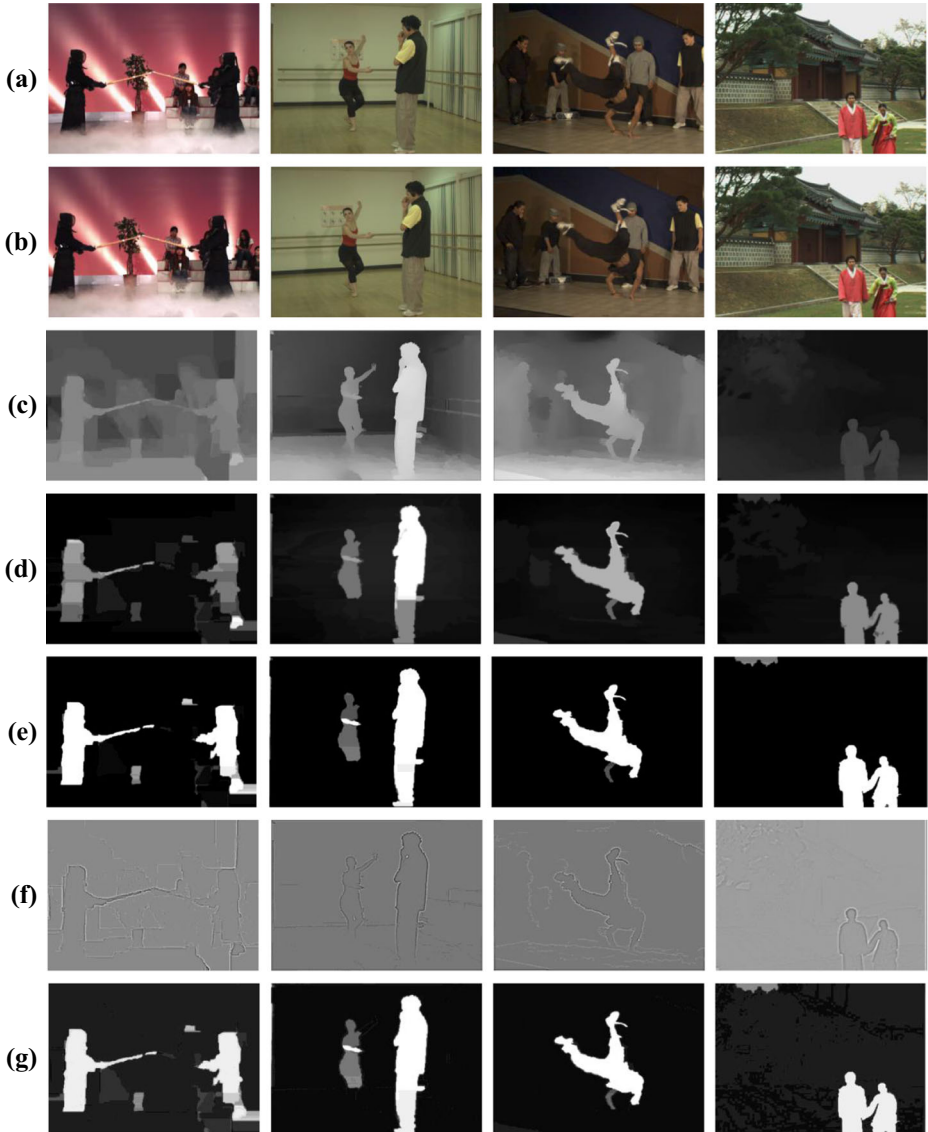
Fig. 2 Depth saliency map estimation. a Left-view image. b Right-view image. c Disparity map. d Preprocessed disparity map. e Foreground saliency map. f Depth edge contrast map. g Depth saliency map
