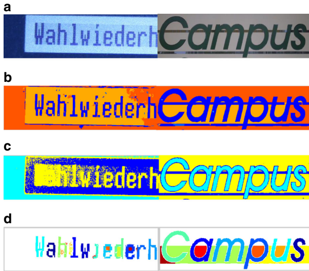
Fig. 9 Examples of initial candidate text line segmentation results. a The candidate text lines. b The segmentation results obtained using multi-layer segmentation. c The segmentation results obtained using GMM-based color clustering. d The selected CCs after overlapped CCs selection
