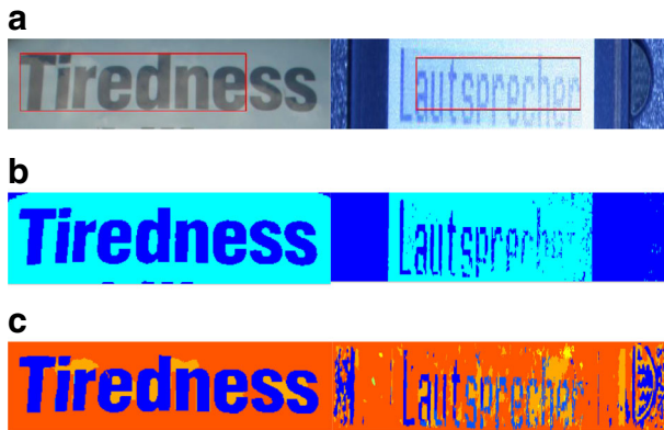
Fig. 11 The recursive segmentation for a text line. a Its area is expanded based on the last time detection result. b The segmentation result using graph cut based segmentation. c The segmentation result using multi-layer segmentation
