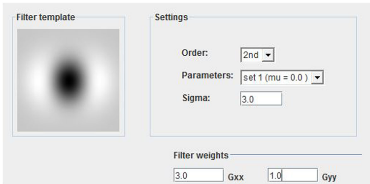
Fig. 3 The different parameters of Steerable filter: The order of the feature template, The smoothness parameters used during the filter optimization, The standard deviation of the Gaussian on which the steerable templates are based and the Weights vector
