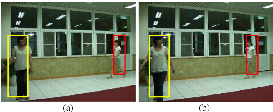
Fig. 14 Two people tracking in indoor environment, particle number: 50
