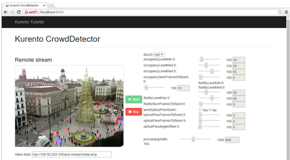
Fig. 7 Web user interface of “Crowd detector” application. It shows a real-time video stream from IP Camera augmented with colors, which depend on the detected level of crowdedness
