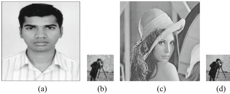
Fig. 10 a, c Watermarked of Photo and Lena Images after JPEG Compression(Q=30) (b, d) Extracted watermarks
