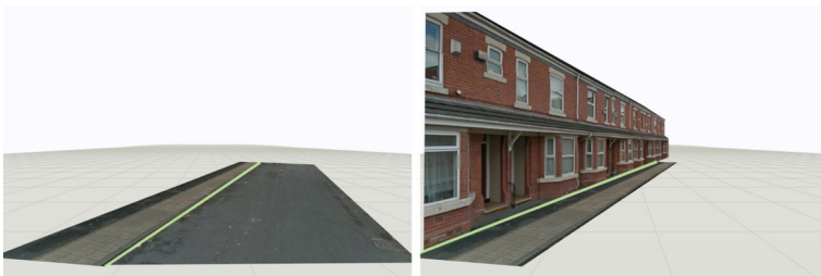
Fig. 10 Guessing the best-suited object class for a sidewalk. The user selects the green edge and the system, depending on the sign of the increment of the X screen coordinate between the two edge endpoints (assuming vertices in counter-clockwise order), automatically selects the road class (left) or the building class (right)
