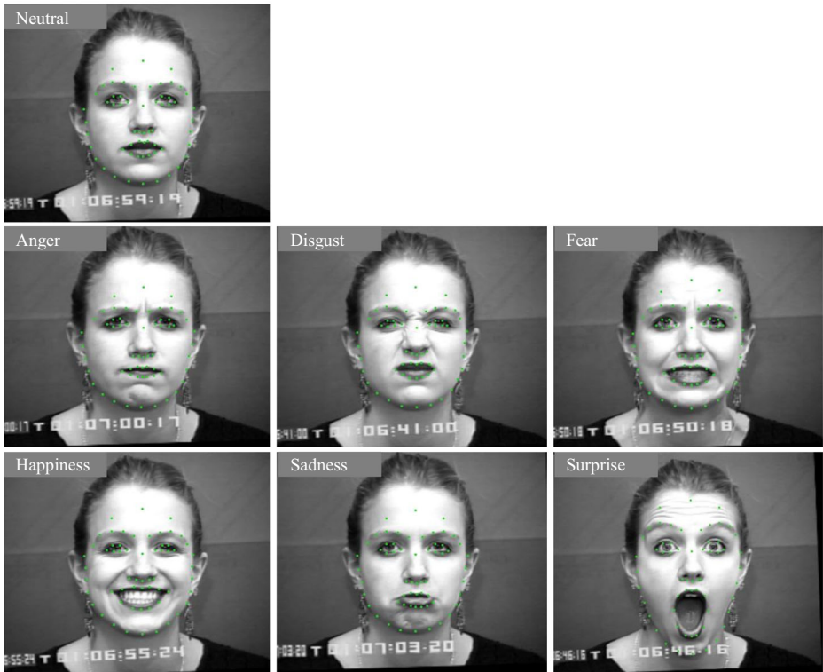
Fig. 2 Facial landmark estimation using regression tree based method presented in [15]. Note that the landmark positions in chin region are located according to eyebrow and eye landmark positions in order to cover chin region
