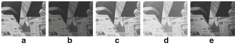
Fig. 8 (a) input image; synthetically illuminated Venus image by (b) multiplicative factor; (c) additive factor; (d) gamma factor; and (e) vignetting effect
