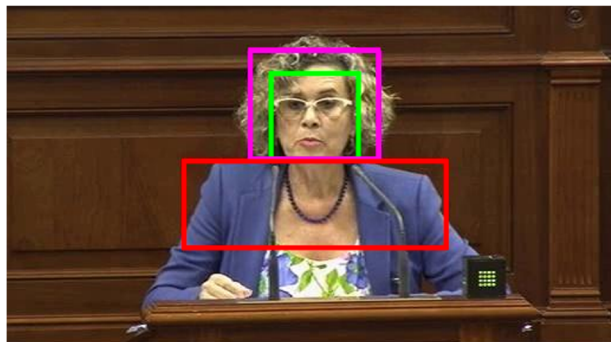
Fig. 4 Areas extracted from each frame to obtain the descriptors of the speaker: magenta bounding box contains the hair descriptor area, green bounding box contain the face descriptor area and the red bounding box contains the torso descriptor area
