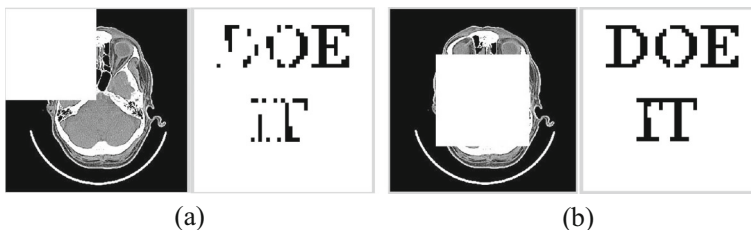
Fig. 23 a 25%Left corner cropped image, Extracted watermark (b) 25%centre cropped image, Extracted watermark
