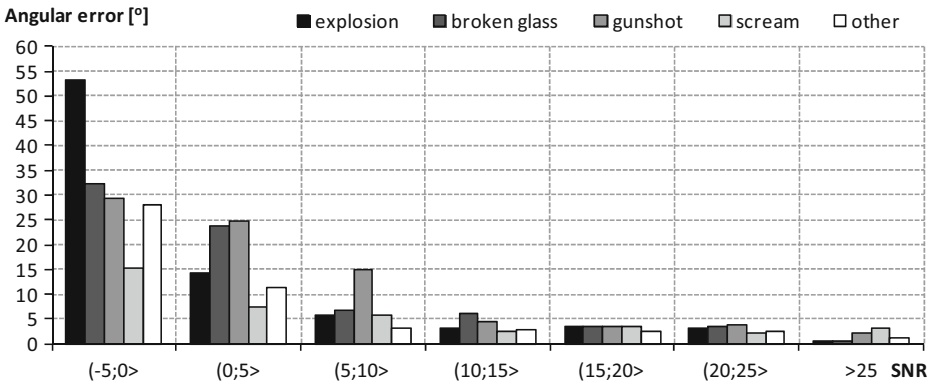
Fig. 18 Localization results (expressed as median values) for all type of noises plotted as a function of SNR values for different types of acoustic events
