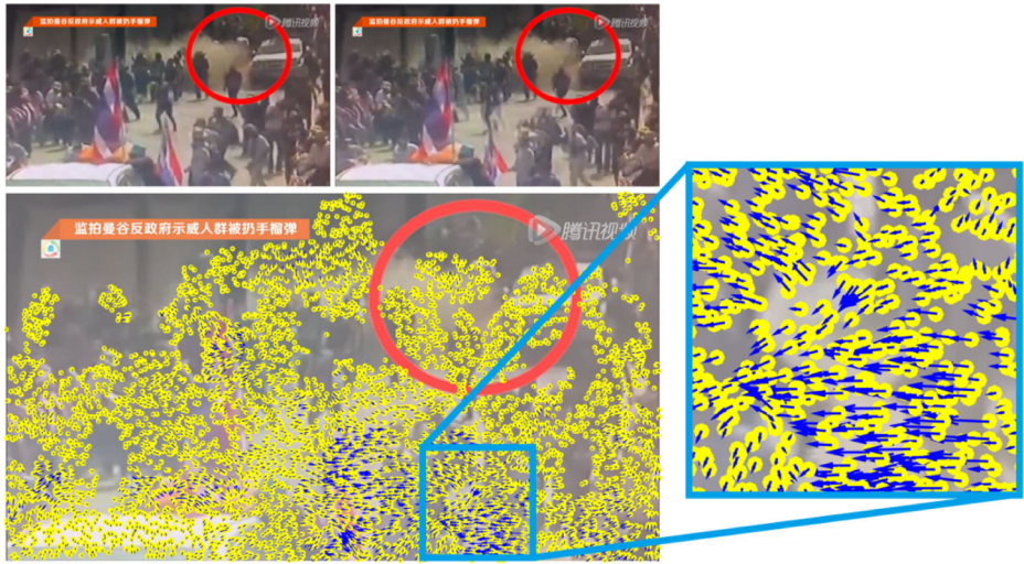
Fig. 3 The up-left images are two continuous frames used to calculate the optical flow. The bottom-left image shows that particles computed from the optical flow cover the motion field. The right shows the enlarged view of the corresponding region
