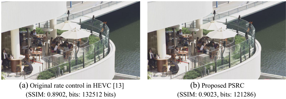
Fig. 1 The reconstructed video frame—“ BQTerrace ”, 17th frame, QP=32 , Low Delay Setting)
