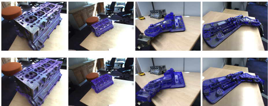
Fig. 13 Registration with a CAD model ( first row ) and with the reconstructed model ( second row ). The 3D mesh is represented in blue
