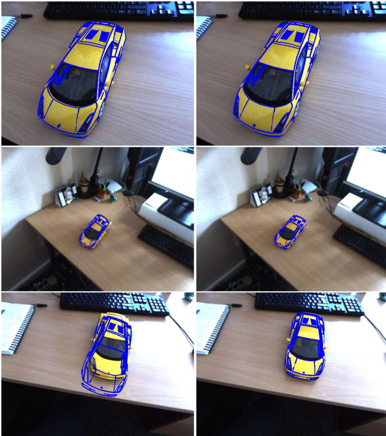
Fig. 7 Localization in a partially known environment composed of a textureless 3D object. Left: results obtained with a model-based tracker similar to the one proposed in [8]. Right: results obtained with a sequential SLAM that uses the proposed LBA_LC&E algorithm
