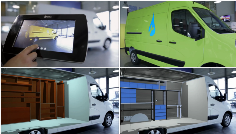
Fig. 16 Augmented Reality on a utility vehicle. Top Left: The tablet used for the experiments. Top right: The original color of the vehicle (white) is changed to green. A specific logo is also added. Bottom: The possible arrangements of the vehicle interior with virtual furnitures
