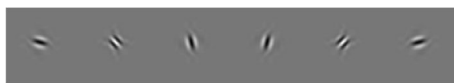
Fig. 1 Impulse responses of six real valued directional wavelets associated with 2-D DTCWT obtained using Eq. (6)
