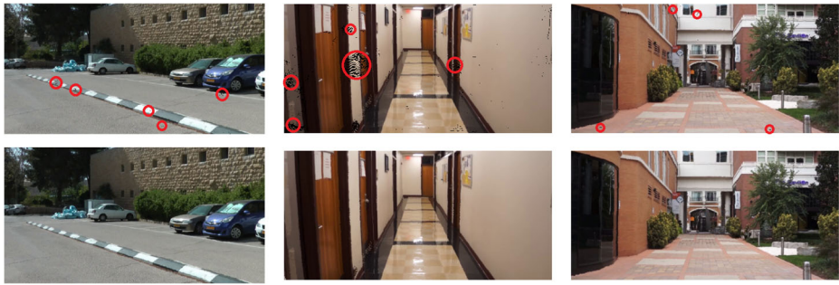
Fig. 3 Performance of image completion algorithm. Top : Frames before image completion. Some pixels are empty (black pixels in red circles ). Bottom : Frames after image completion. All pixels get appropriate values
