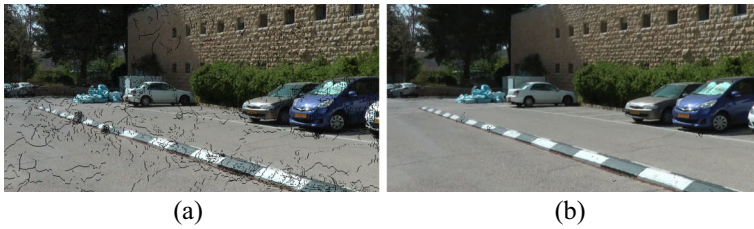
Fig. 2 Performance of weighted average algorithm in frame warping. a Result using rounded values. Many pixels remain empty. b Result using weighted average values. Most pixels are filled
