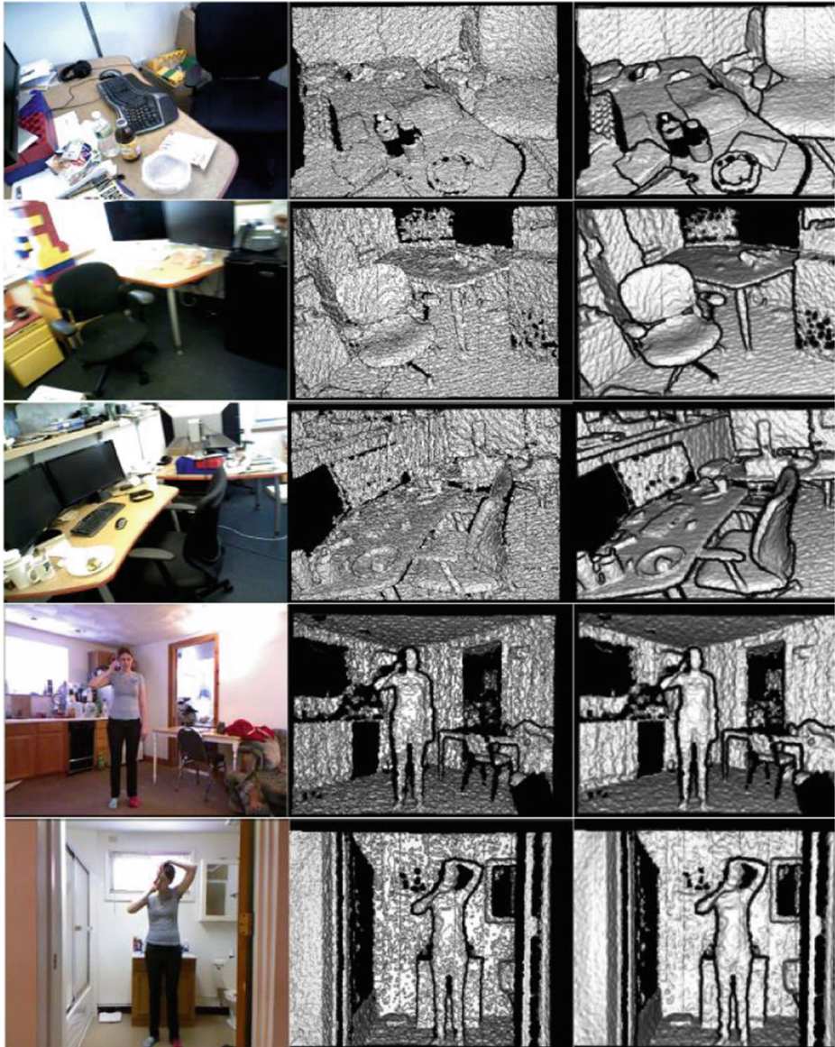
(a) Input RGB image (b) Given noisy depth from Kinect (c) Our approach
