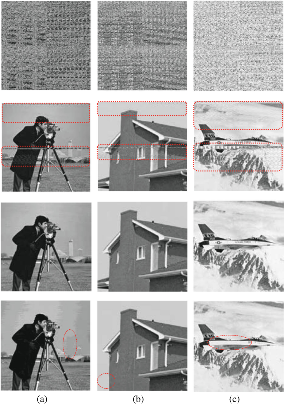
Fig. 3 Attacks on the ESC scheme watermarked images: (a) cameraman, (b) house and (c) jet-plane. From top, 1 st row: Counterfeiting Attack 1 (entire blocks); 2 nd row: Counterfeiting Attack 1 (selected blocks); 3 rd row: Counterfeiting Attack 2; and 4 th row Counterfeiting Attack 3
