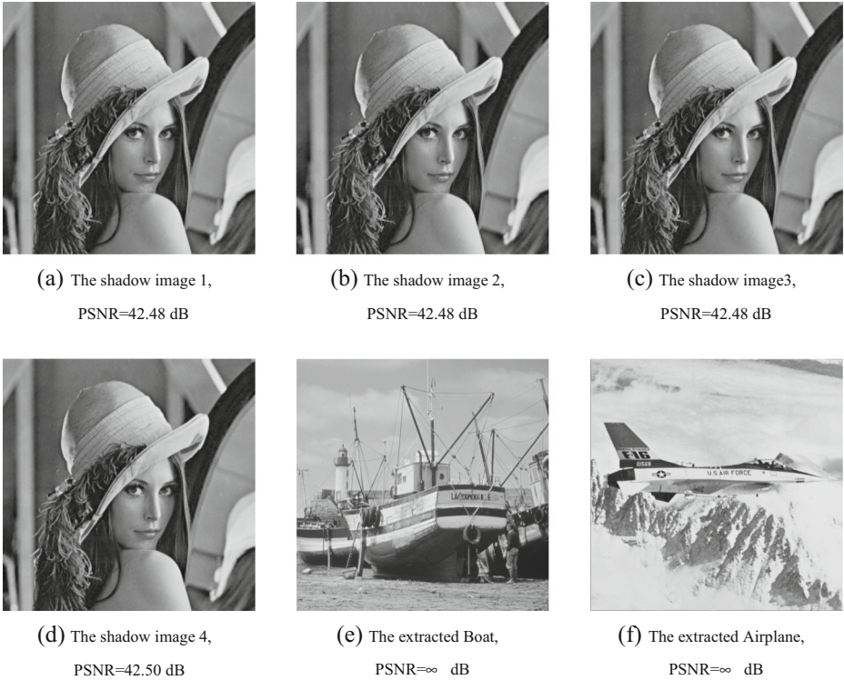
Fig. 5 The results of Lena, for a monotone access structure, q=7 . a The shadow image 1, PSNR=42.48 dB b The shadow image 2, PSNR=42.48 dB c The shadow image3, PSNR=42.48 dB d The shadow image 4, PSNR=42.50 dB e The extracted Boat, PSNR=∞ dB f The extracted Airplane, PSNR=∞ dB
