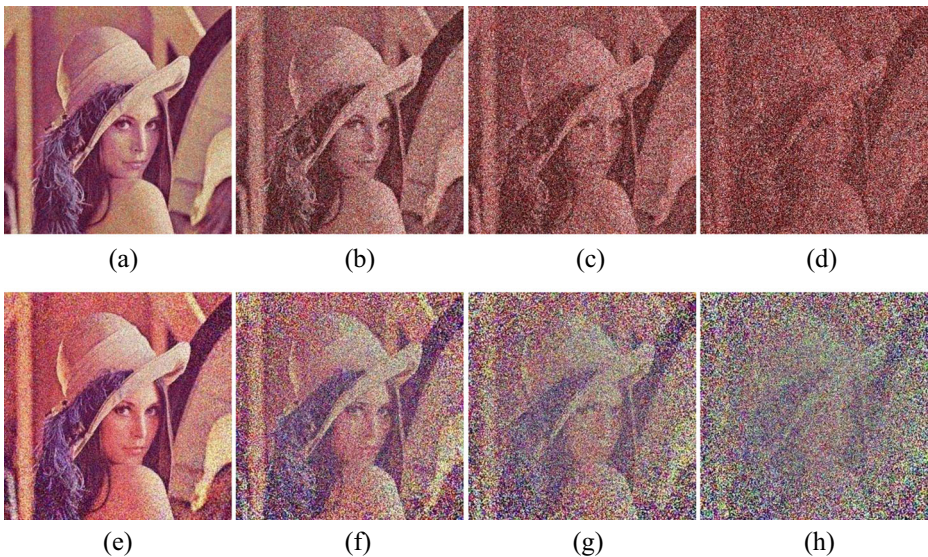
Fig. 8 Decrypted images by RPFrDCT with different Gaussian noise intensities of (a) 10, (b) 30, (c) 50 and (d) 100; Decrypted images by RPFrMT [29] with different Gaussian noise intensities of (e) 10, (f) 30, (g) 50 and (h) 100
