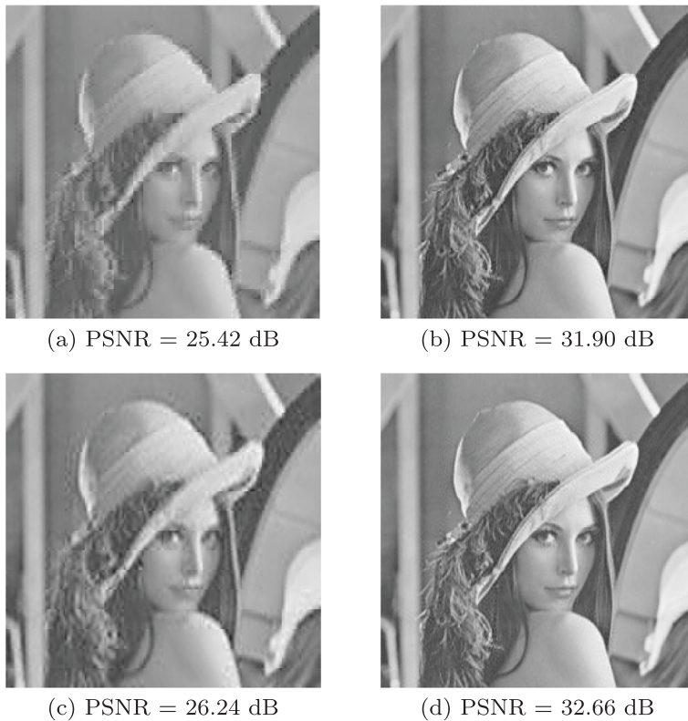
Fig. 9 Simulation results for Lena image with block DCT a MR = 0.1, 8 \times 8 block b MR = 0.4, 8 \times 8 block c MR = 0.1, 16 \times 16 block d MR = 0.4, 16 \times 16 block
