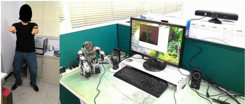
Fig. 1 Kinect-based gesture command recognition using proposed HMM incorporated with an UA scheme for NUI designs of humanoid robot imitations
