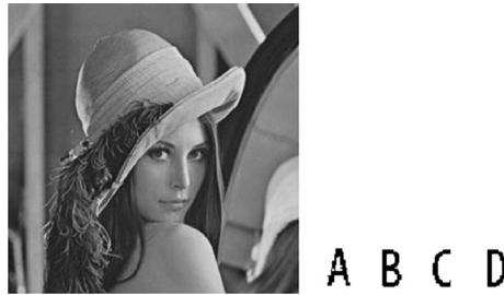
Fig. 4 MWOD-watermarked Lena image with 4 watermarks embedded. PSNR=46.096 dB. 4 Extracted watermark (Right)
