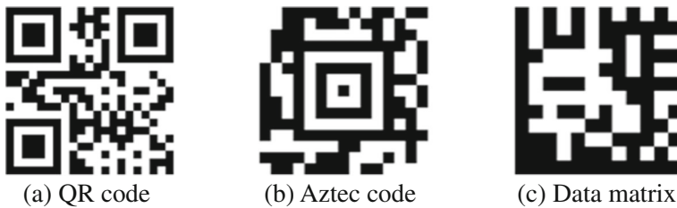
Fig. 2 Examples of various barcode types (each of these barcodes has the same content: AUT)
