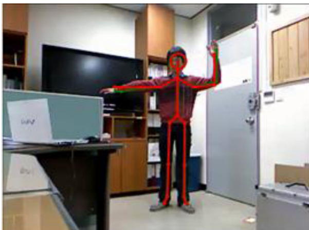
Fig. 4 An example of two overlapped trajectories: the green is the reference motion and the red is the practice one
