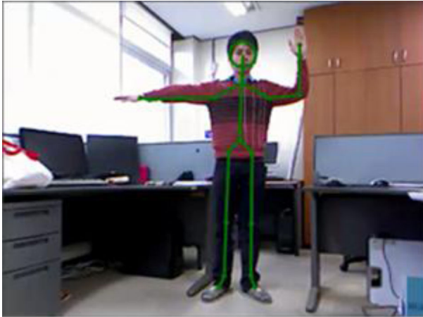
Fig. 3 Human body image overlapped with the joints and skeleton obtained from the Microsoft Kinect system
