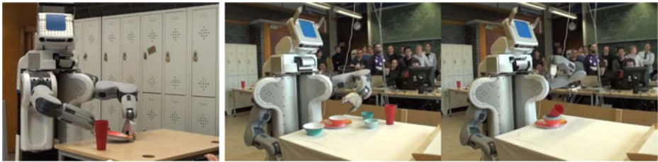
Fig. 3 PR2 is clearing up tables with a cart ( leftside : stacked homogeneous plates and rightside : stacked heterogeneous plates, bowls, and cups)
