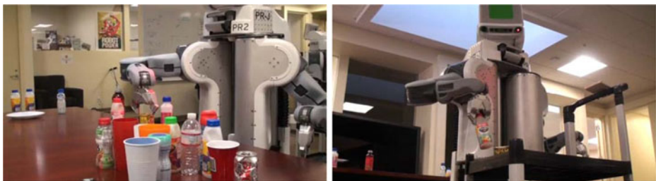
Fig. 2 PR2 can reach for a variety of bottles, grasp, and places them on a cart using its 'Pick and Place' operation based on the cloud resources
