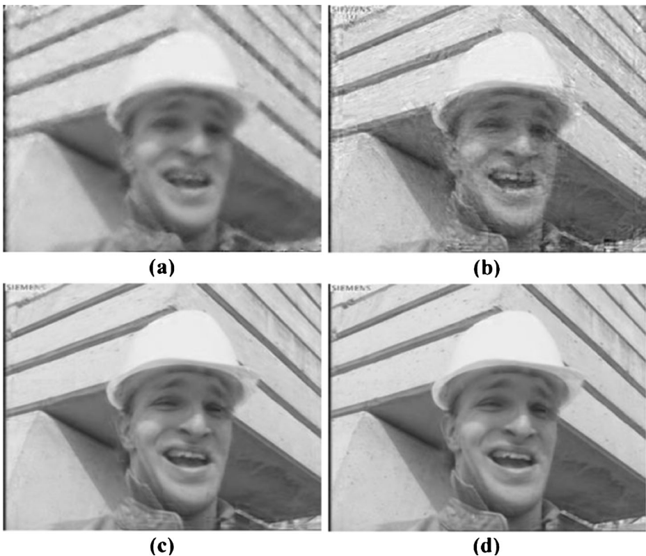
Fig. 12 Reconstruction of frame 15 of Foreman sequence with CS-subrate = 0.1: a Dir-BCS-SPL, PSNR = 26.83 dB b MH-OMP, PSNR = 26.93 dB c MH-Tikhonov, PSNR = 33.31 dB d MS-wEnet, PSNR = 35.86 dB
