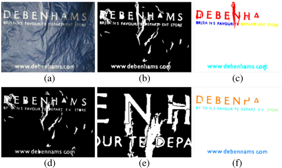
Fig. 3 a The original image. b Detected MSERs. c Detected text lines by using MSERs as in (b). d Image mask integrating MSERs and canny edges. e Magnification of part of (d). f Detected text lines by using MSERs as in (d)
