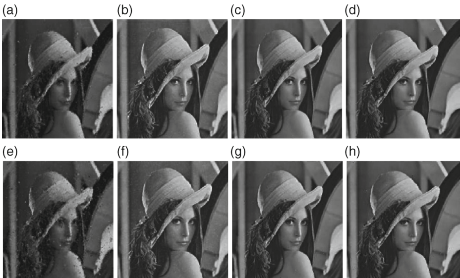
Fig. 11 a–d Restored 20 % corrupted Lena image by ACWM[8], DWM[11], FTPID[2] and the proposed method respectively; e–h Restored 40 % corrupted Lena image by ACWM[8], DWM[11], FTPID[2] and the proposed method respectively
