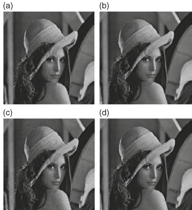
Fig. 10 a–b Restored 20 % corrupted Lena image by JWD [25] and proposed method respectively; c–d Restored 40 % corrupted Lena image by JWD [25] and proposed method respectively
