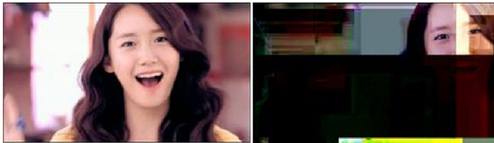
(c) Original and distorted frame at packet loss 0.05% and jitter 48ms (SSIM=0.958)
